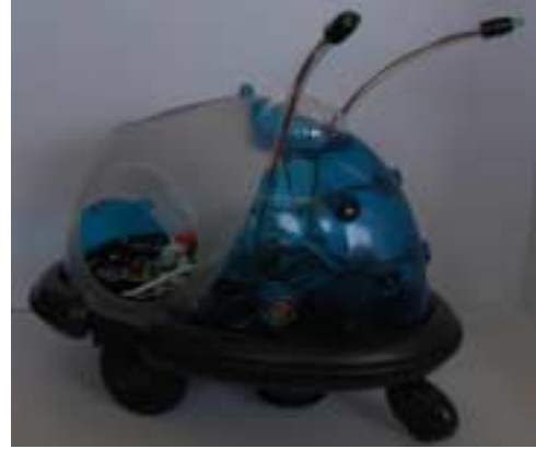
Figure 1. Real Robots "Cybot" Mechatronics showing the ultrasonic proximity sensors.
